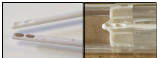
Figure 7: HM-JACKarc collection probe dimples, with and without sample, and collection device septum.
